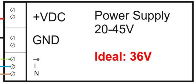
Ideal power voltage ist 36V DC. Maximum allowed is up to 50V but not recommended as it will shorten the devices lifespan. Use 36V whenever possible!
